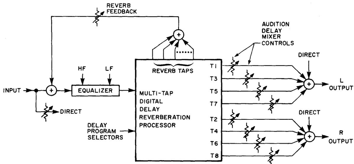
Fig.4: Multi-Tap Digital Delay Block Diagram.
